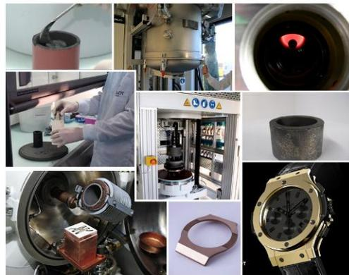
The magic of the scratch-resistant “Magic Gold” lies in its ability to withstand pressure up to a hardness of 1000 Vh1, far higher than standard 18-carat gold (400 Vh1) and quenched steel (600 Vh1). This means that for a Big Bang Ferrari with super gold armor, only a diamond with a hardness of 2000 Vh1 could leave a scratch of any kind on its surface.
