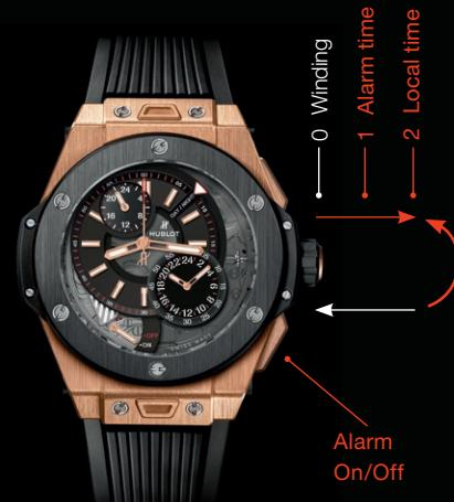
1. Turn the crown a quarter-turn anti-clockwise. The crown is in the 0 position, which enables the watch to be wound manually. It takes 45 turns of the crown to fully wind the watch, i.e. for the 72-hour power reserve.
